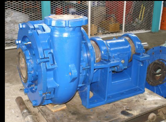
ALL METAL PUMP RECONDITIONING
